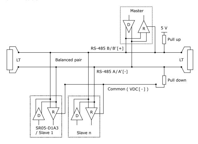
**Figure 5.11.1** Typical topology of a two-wire RS-485 network, figure adapted from: Modbus over serial line specification and implementation guide V1.02 (www.modbus.org). The power supply is not shown in this figure.
