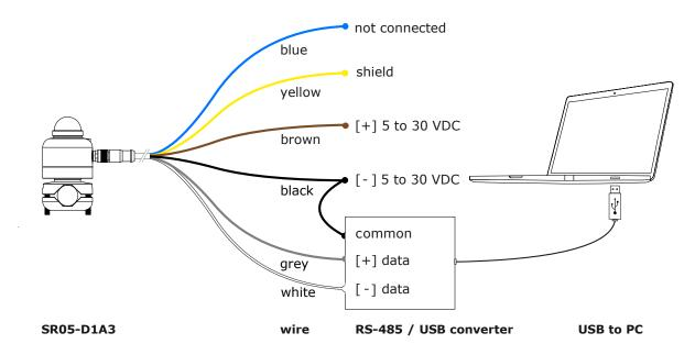
Figure 5.13.1.1 Connecting SR05-D1A3 to an RS-485 to USB converter and a PC
