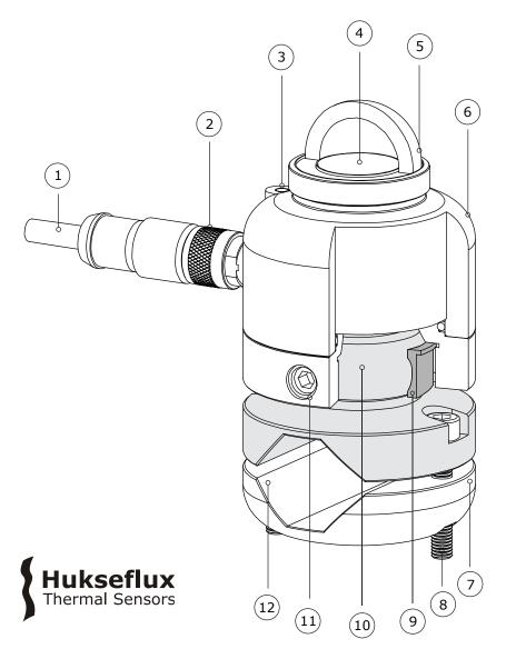
**Figure 2.1** Overview of SR05: shaded areas in exploded view show ball levelling mount and shim
