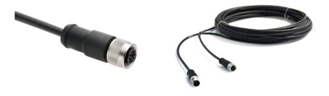
**Figure 9.1.1** On the left the SR05 cable with M12-A female connector on sensor end. The cable is non-stripped on the other end. Its length is 3 metres standard and available in 10 and 20 metres too. On the right Hukseflux extension cable with connector pairs, with male and female M12-A connectors, available in 10 and 20 metres.
