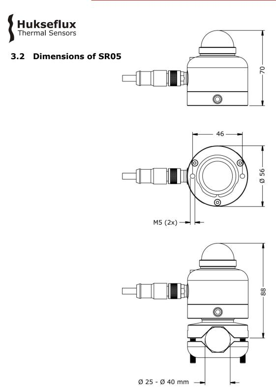
**Figure 3.2.1** Dimensions of SR05 in  $\times$  10<sup>-3</sup> m. The bottom drawing shows the height of SR05 combined with its optional ball levelling mount and the tube diameter required for use with SR05's optional tube mount. M5 mounting bolts and the countersunk set screw require a 4 mm hex key for mounting and levelling.
