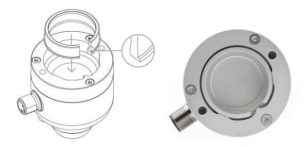
**Figure 5.5.1** Line drawing indicating placement of the aluminium shim and photo showing the shim properly positioned in the centre of SR05's bottom plate. Note the position of the protruding ledge when placing the shim.
